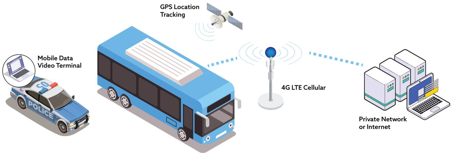
The MBTA has two departments with live system access: the Operations Control Center (OCC) and MBTA police dispatch, along with transportation executives. The unique dual-mode radio system provides both Wi-Fi and Verizon 4G LTE wireless connectivity, a crucial advantage. This versatility allows multiple ways to access video, enabling real-time emergency responses and investigations.
